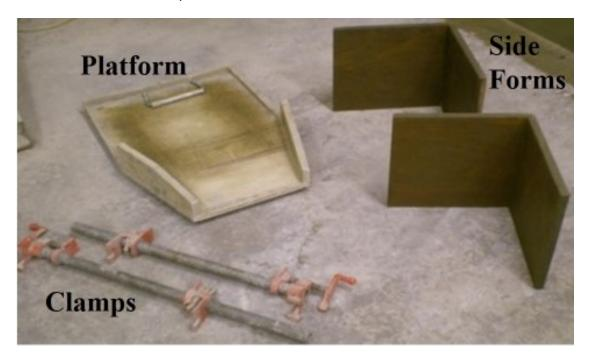
Figure 1 Each Component of the Box Test
