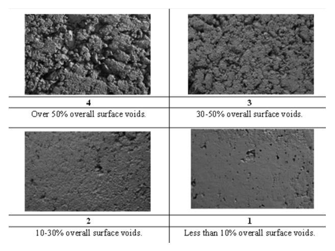
Figure 4 The Box Test Ranking Scale
